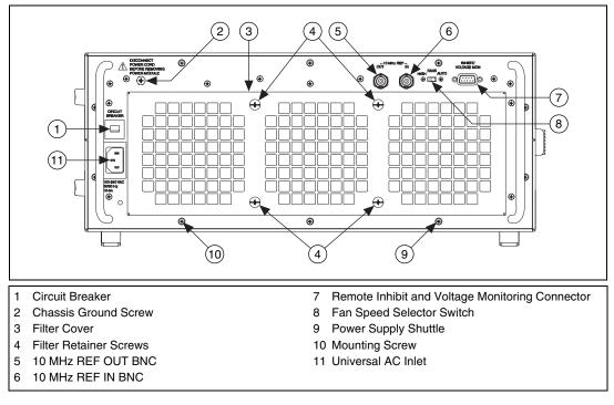
Figure 1. PXI-1045 Power Supply Shuttle Rear Panel
